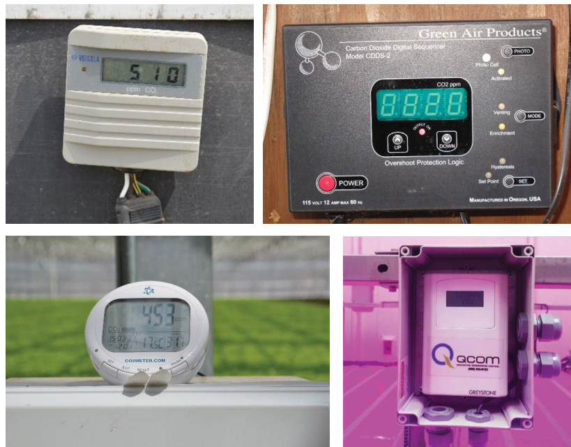
Figure 1. Examples of digital carbon dioxide (CO 2 ) meters and controllers. Some meters can be connected to a computer to monitor and maintain set point maximum and minimum carbon dioxide levels. Photo by Roberto Lopez.
