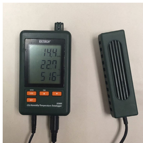
Figure 2. An example of a hand-held CO 2 meter that can be used to take instantaneous CO 2 readings. This meter also displays air temperature and relative humidity readings.
